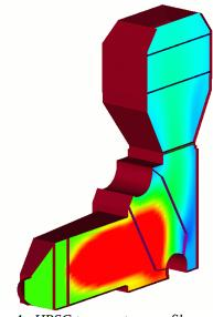
*Figure 4 - HRSG temperature profile*
