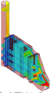
Figure 3 - HRSG velocity profile
