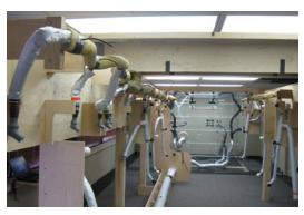
Figure 2 -ASC was contracted to build a physical model of the cabin ducting system and balance flow.
