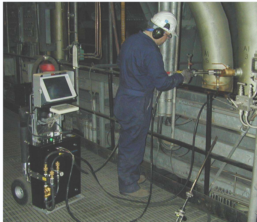
Coal pipe testing with Advanced Coal Flow Measurement (ACFM) device
