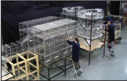
Figure 4. Physical flow model of a power plant dry scrubber and baghouse system
