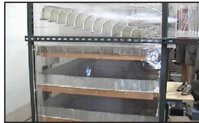
Figure 5. Smoke flow through an SCR physical model
