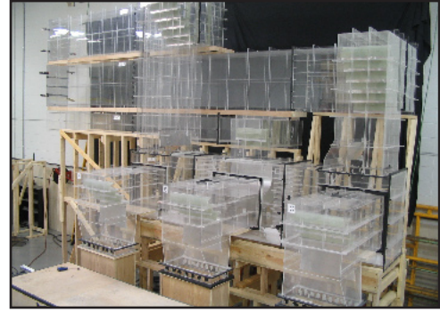
Figure 6. Comparison of CFD and physical model results for an FGD duct system where flow from 3 units (1,750 MW total) combine to feed 3 new booster fans (CFD pressure drop 1.19 IWC; Physical pressure drop 1.27 IWC)
