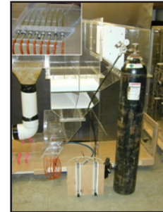
Figure 11. Physical model testing of ammonia injection in an SCR via tracer gas simulation
