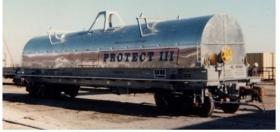
The railcar covers shown above are used to enclose and protect large steel coils while in transit. The covers are lifted off by crane and then stacked when the coils reach their destination. ASC's analyses ensured that the structure of these covers would hold up under these load conditions.
