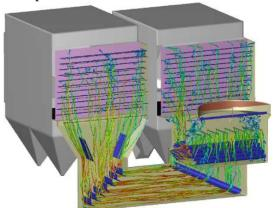
CFD model tracks the trajectory and velocity of carbon particles from the lances to the ESP.
