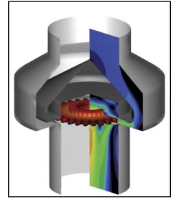
*CFD* model of a gear in an intensive quench fixture.
