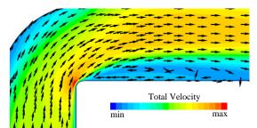
Figure 1: With no vanes, a turbulent, recirculating flow region exists.
