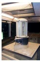
signing the turbine support structure. The extent of the turbine wake was also measured. This data will be used to set the spacing on the array of turbines.
