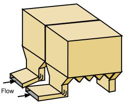
Figure 1. ESP Geometry
