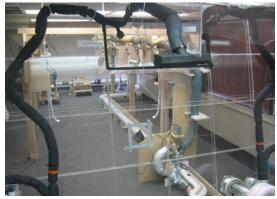
bulkheads, that problem would not have been identified through a more traditional on-aircraft test program. Boeing is now working with their supplier to update those duct components.
