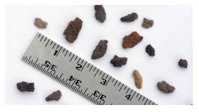
burned, and furnace flow patterns. As seen in the figure above, LPA can often be characterized as particles greater than 5 mm in size. This type of ash can quickly plug air preheater baskets and SCR catalysts resulting in significant increases in pressure loss that require frequent operation at reduced load and costly outages to perform cleaning.
