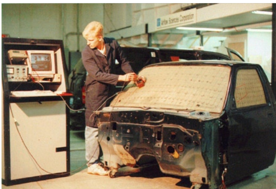
Figure 1 - Test apparatus for measuring air velocity on windshields
