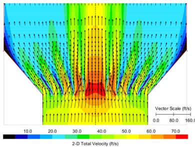
Figure 3 - Velocity profile in ESP inlet expansion
