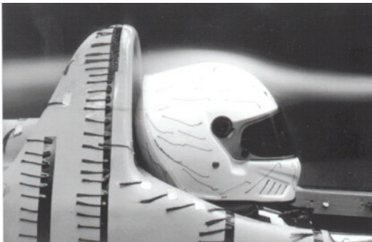
Figure 1 - Visualization of flow field around new helmet design
