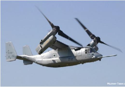
*Figure 1 - Bell-Boeing's V-22 Osprey aircraft developed for the US Military. Designed for short and vertical take-offs with long-range, cruise performance.*
