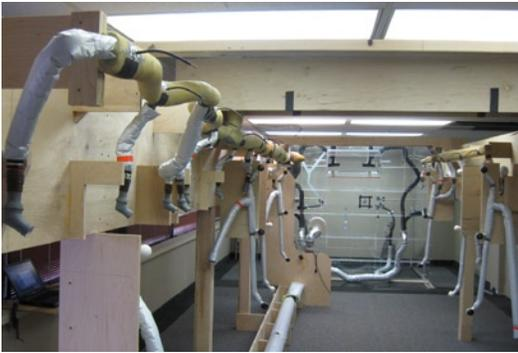
*Figure 2 -ASC was contracted to build a physical model of the cabin ducting system and balance flow.*
