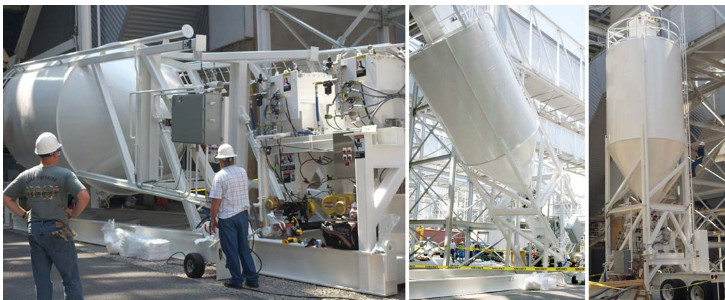
Figure 8: A self-erecting portable sorbent storage silo moved into position and then using self-contained hydraulics rising into a fully erect posture.
