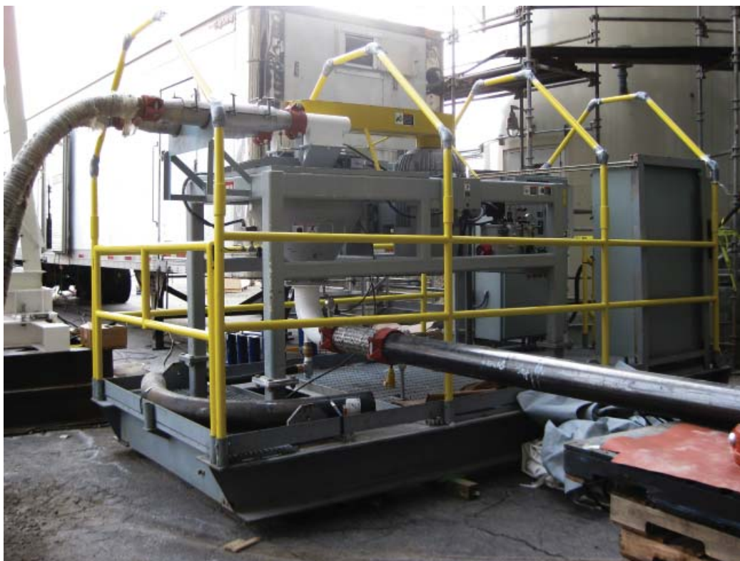
Figure 10: An example of an in-line blow through variable speed rotary pin mill used to improve removal of SO 2 and SO 3 .
