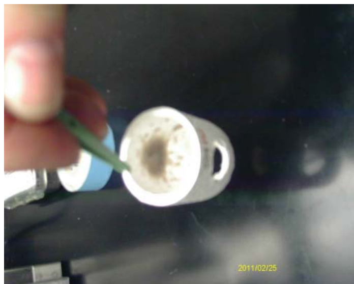
Figure 18: Pre-cutter liner from FGD outlet test
