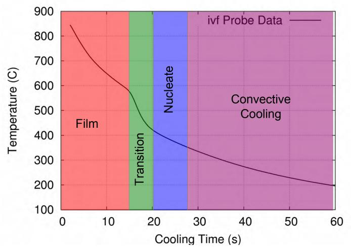
Divide surface heat transfer model up into typical boiling regimes.
