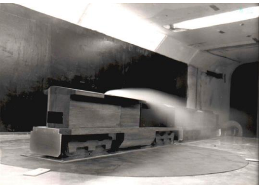
Figure 4: Wind Tunnel Test of Locomotive at 1:15 Scale
