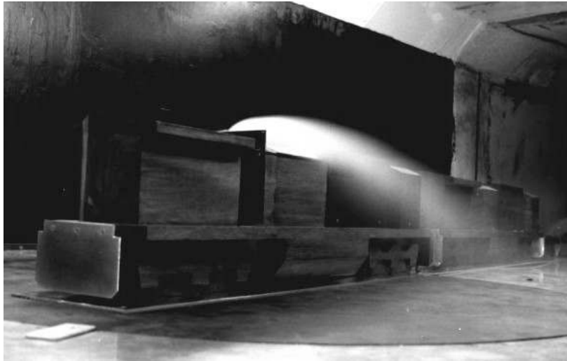
Fig. 15. Diesel Exhaust Plume Behavior: 1/15-Scale Wind Tunnel Test, Yaw Angle = 10°, Long Hood Forward, Baseline Exhaust System
