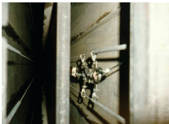
Figure 5. Vane Anemometer Assembly for Weighted Wire ESPs
