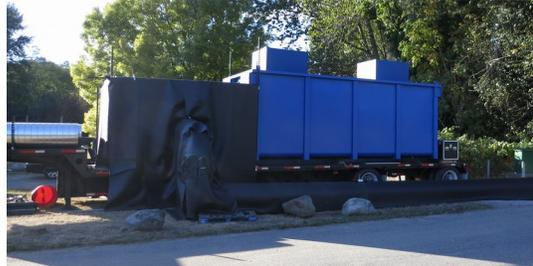
Figure 1: Portable Scrubber System
