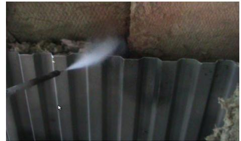
Figure 2: Smoke wand testing method
