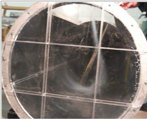
Figure 3: Smoke visualization in the physical model confirmed the flow swirl patterns in the stack that were identified in the CFD model.
