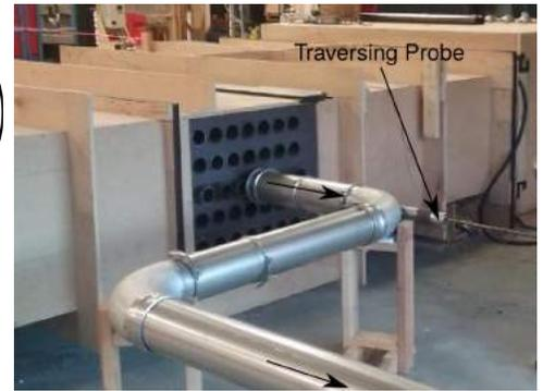
Figure 5: The active tube outlet view shows the traversing thermocouple probe, used to quantify the temperature distribution through the tube length.
