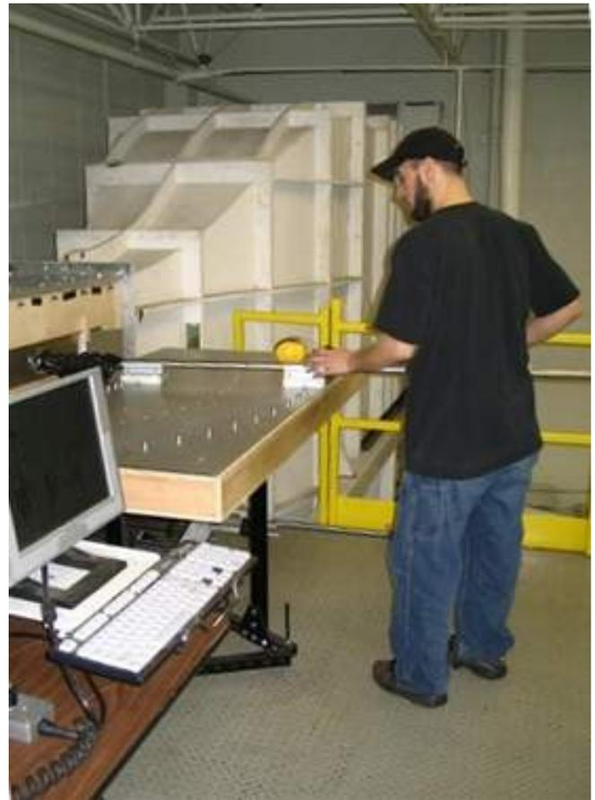
Figure 4: Both the Flow Bench and wind tunnel are used to calibrate a variety of velocity probes.
