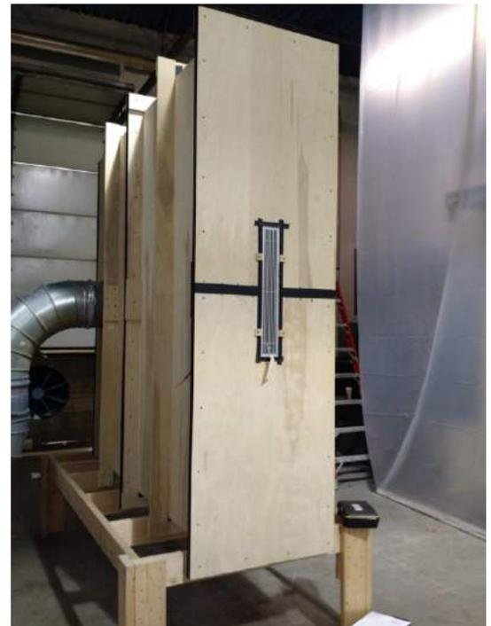
Figure 2: The various grilles were placed in this pressurized supply plenum, which included straighteners and perforated plates to ensure even flow at the register.
