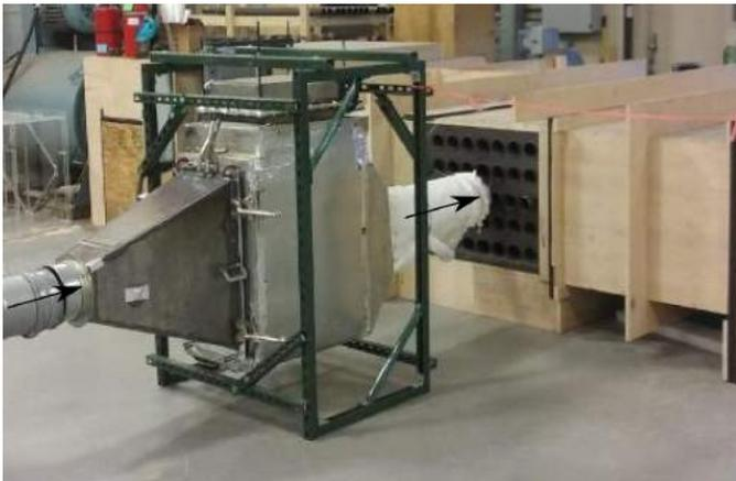
Figure 2: An air heater provides hot air to the active tube (inlet view), located at the center of the tube bank array.
