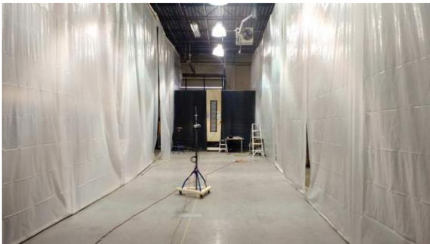
Figure 3: Curtains were installed beyond the furthest location of the movable probe stand to ensure accurate measurement of the throw distance from the grille.
