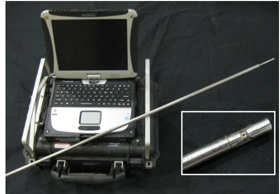
Figure 11. 3D Probe and 3DDAS Measurement System
