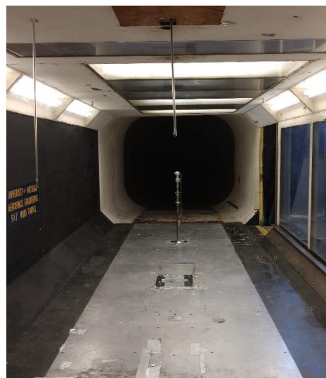
Figure 6. PM10 Probe in UofM Test Section
