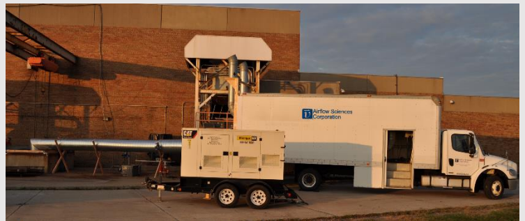
ASC's Mobile Extractive Sewer Sampler houses all the equipment necessary for efficient mobile sewer testing
