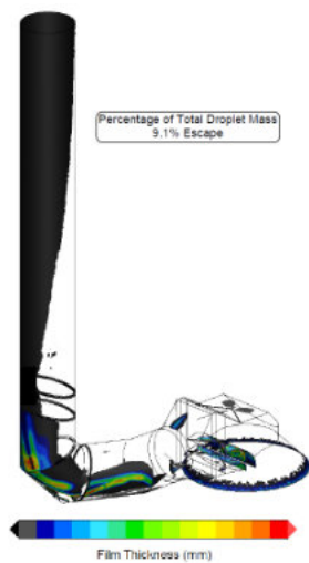
Figure 13: 9.1% of total droplet mass escapes
