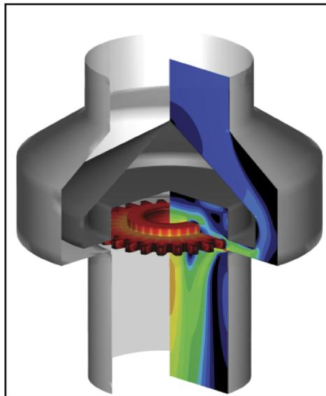
*CFD model of a gear in an intensive quench fixture.*
