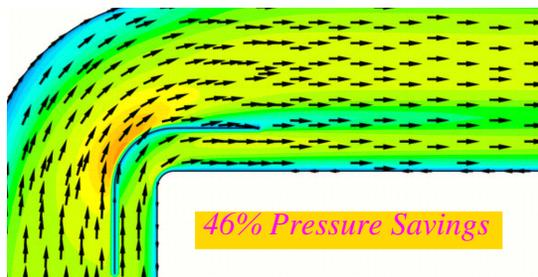
Figure 2: Optimized turning vanes result in a smooth, low turbulence attached flow regime.
