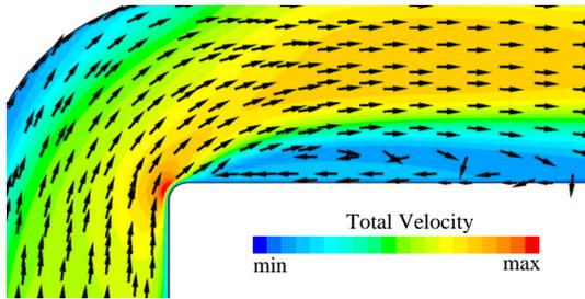
Figure 1: With no vanes, a turbulent, recirculating flow region exists.
