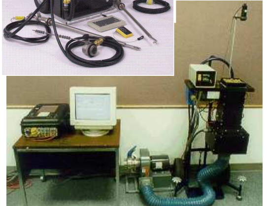
Laboratory scale pet food dryer
