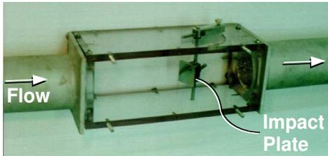
Figure 3. Test Fixture to Determine Particle Build-up Characteristics
