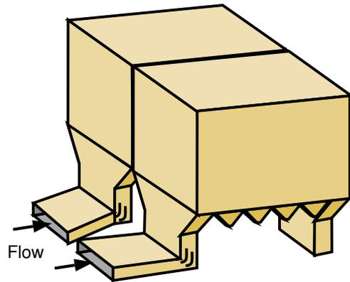
Figure 1. ESP Geometry
