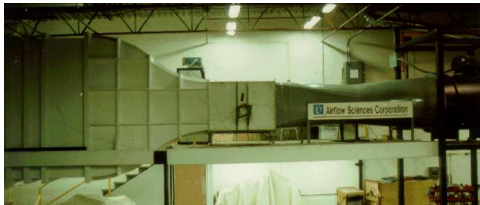
ASC's 17"x34" Subsonic Wind Tunnel
