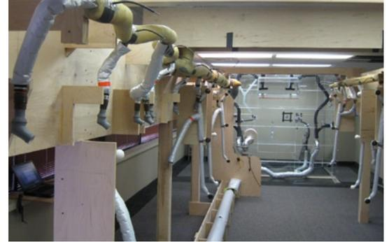
through the system. One unexpected outcome from the test program was the identification of several duct components that were not robust enough to withstand the negative pressures that would occur during certain operating modes. As those ducts would be located within enclosed
